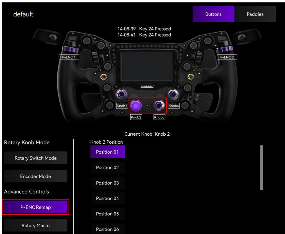
Switch the selected knob to "Position 01", rotate P-ENC 1, and the log will show that Key 23 or 24 is pressed. Rotate P-ENC 2, and the log will show that Key 25 or 26 is pressed.
