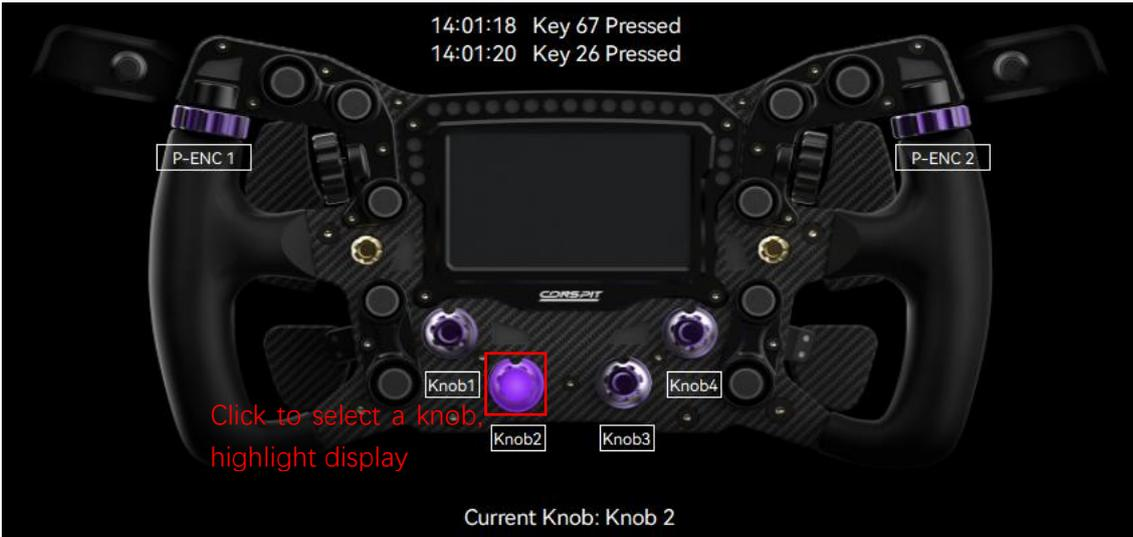
[Knob 1] and [Knob 4] can be set to use either [Rotary Switch Mode] or [Encoder Mode].
