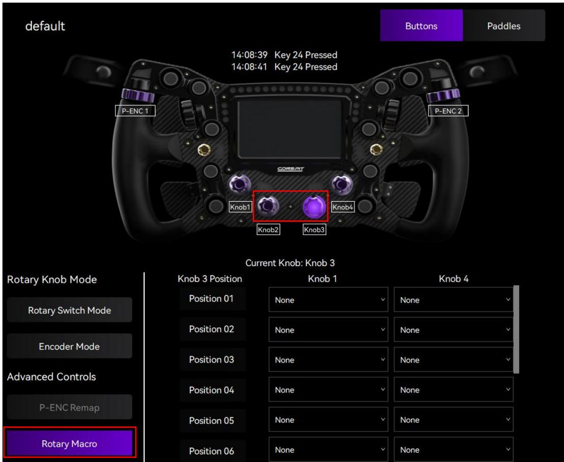
For example: Select Knob 3, click on "Rotary Macro", and then click on the dropdown menu to set the corresponding positions of Knob 1 or Knob 4 for each position of Knob 3 in sequence. After completing the settings, rotating Knob 3 with the configuration done will simultaneously trigger the Keys of Knob 1 and Knob 4 that are mapped to the current position of Knob 3.
