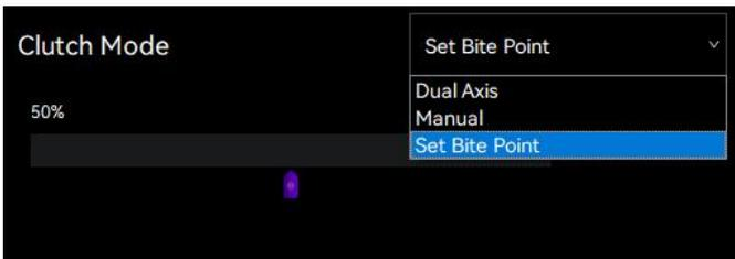
Drag the purple slider located below the "Clutch Mode" display section to adjust the bite point.
