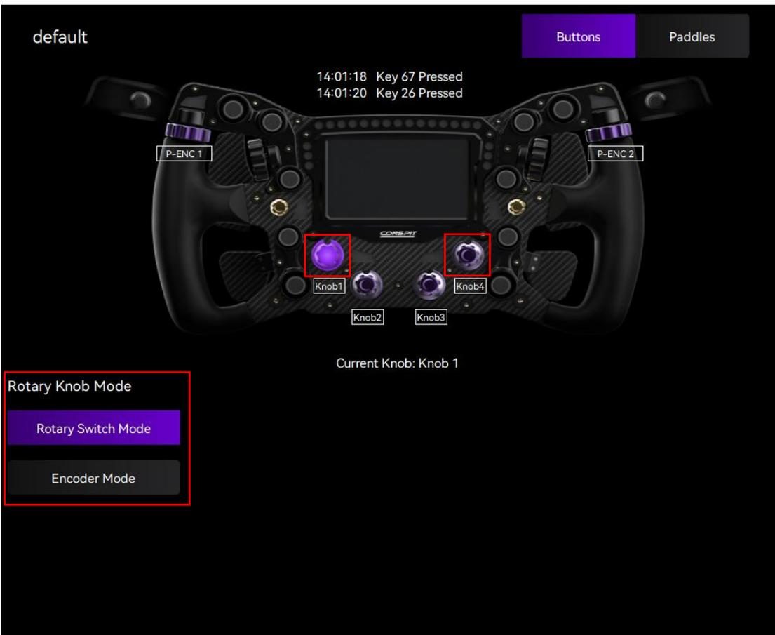
[Knob 2] and [Knob 3] can additionally utilize advanced functions, including [P-ENC Remap] and [Rotary Macro].
